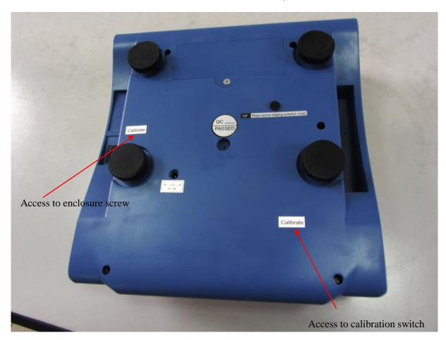
Figure 9 Sealing of EP100 / EP110 / EP200 / EP210.
